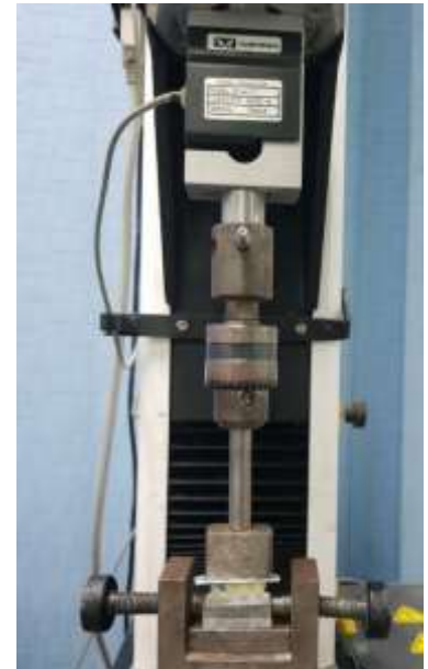
Figure (7): Sample in Universal Testing Machine
