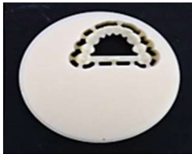
Figure 4: "Milling procedure": A sample in puck after milling completion.
