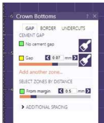
Figure 2: “Designing software setting”: zero gap distance between the Locator metal housing and the fitting surface of the prosthesis.
