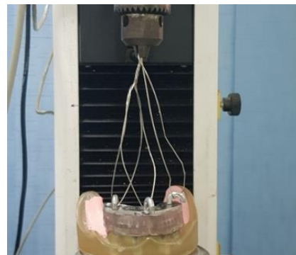
Figure (6) Metal pickup on epoxy model during measuring retention
