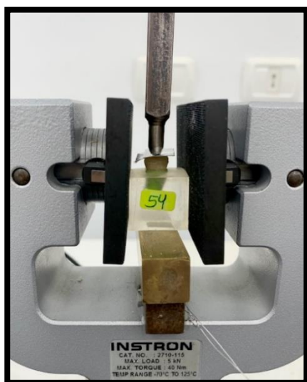
Figure (4): Fracture resistance test using Instron universal testing machine
