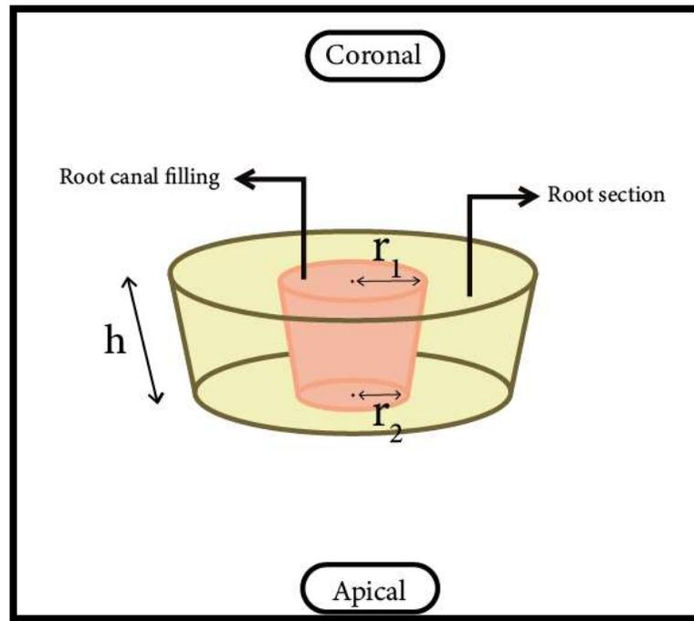
Figure 1: Diagram showing measurements for calculation of adhesion surface area.
