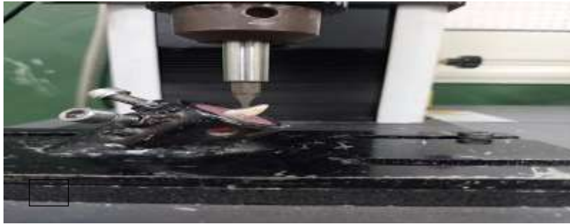
Figure (2): Fracture resistance test
