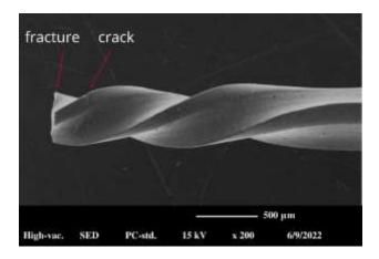
Figure 2: Edge file cracks and fractures after preparing 9 canals in the CAC group.
