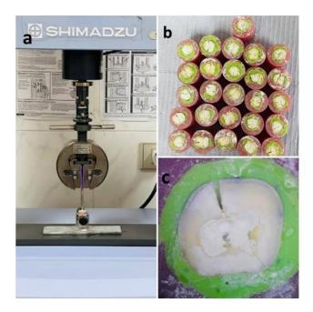
Figure (5): (a) sample within the universal testing machine (b, c): samples after the applied force with the vertical fractures occurred.
