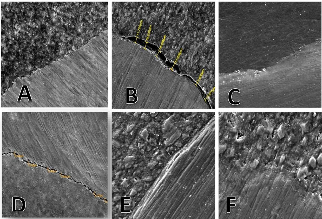
**Figure 3:** Representative Stereomicroscopic images of: (A) Continuous margin of Tetric Evoceram Bulk fill. (B) Non continuous margin for Tetric EvoCeram. (C) Continuous margin for Filtek posterior (D) Non continuous margin for Filtek posterior. (E) Continuous margin for Activa. (F) Continuous margin for Sonic Fill.
